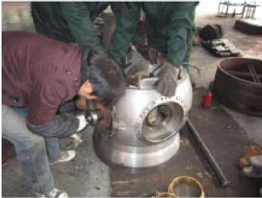
Runner hub is in process of fixing brass bush.
