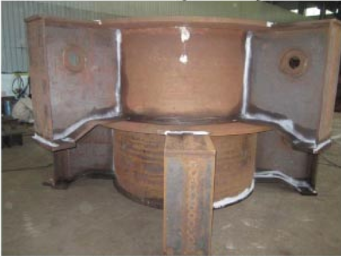
Three upper brackets are annealed. MT is finished.
