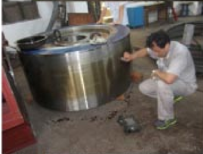
UT testing on end face and around body of a magnetic yoke, the test result is acceptable.
